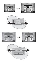
2. Then sharpen the image by rotating the FOCUS ring.
